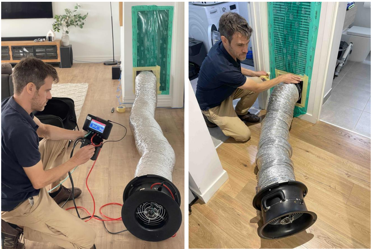
Figure 36 Duct testing setup
